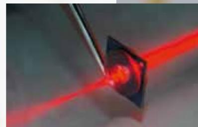
Adaptive lens with piezo actuator
