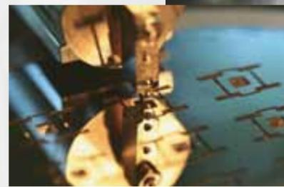
Wafer-level microtensile test
