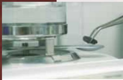
Gravimetric determination of density
