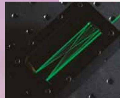
Multireflection cell for optical gas measuring technologies
