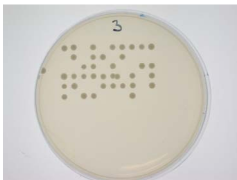
Fig.7: Seeding single yeast cell array on culture media. Deposited spots containing yeast cell grow to form colonies after 72 hours incubation.
