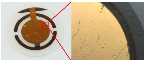
Fig. 1: Sensor of QCM100, coated with about 2 \mu\text{m} thick surface-attached and cross-linked polymer hydrogel
