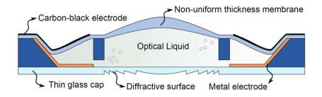
A conceptual depiction of a hybrid tunable aspherical lens with an integrated electroactive polymer actuator. While this approach is an option, several other actuation techniques will also be explored in the project.
