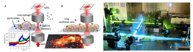
Left: Optically trapped and non-trapped particles fluctuate nearby living cells. Trapped particles are moved toward the cell membrane and its positions fluctuations (3D trace) are recorded in 3D at 2 MHz temporal resolution via quadrant photo-diodes (QPDs). Bottom insets: microsecond nanometer position traces of the particles defined by thermal and cellular forces. Label-free ROCS-superresolution image of a macrophage with many 200 nm particles. Right: Photo of ROCS setup.
