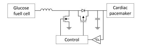
The task of this master thesis is the development of an integrated dc-dc converter which is able to operate under ultra-low power and ultra-low voltage conditions. Moreover, a lowpower control circuit is to be developed in order to achieve high efficiency since only some microwatts are transferred from the glucose fuel cell to the cardiac pacemaker. A low power consumption of the circuit is thus of utmost importance.
