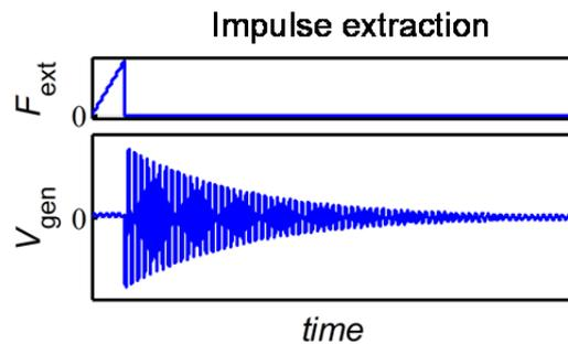
Figure 2: External force (top) and open-circuit voltage
